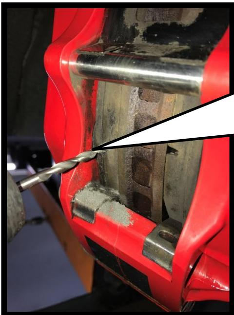
Now slightly enlarge the diameter of the hole with the 4.5 mm drill so the sensor gets a tight fit into the hole .
