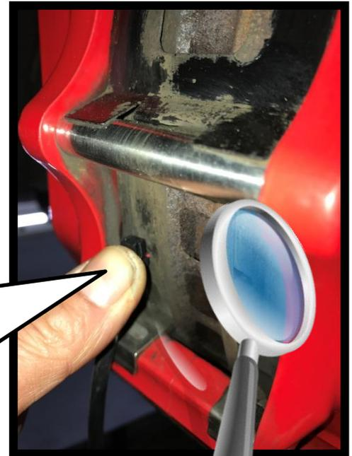
**UK** The sensor needs to be Manually installed and pressed by hand into the hole until it is secure
