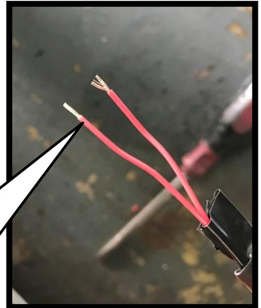
🇬🇧 Remove +/- 15 mm of wire insulation from the V-Maxx Autosport Brake Pad Wear Indicator
