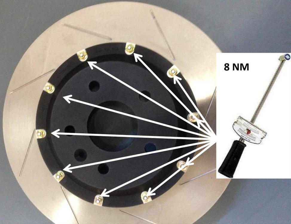
Apply Loctite on the M5 x 30 Allen screw and M5 locking nut
