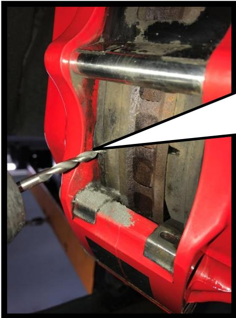
**UK** Now slightly enlarge the diameter of the hole with the 4.5 mm drill so the sensor gets a tight fit into the hole .
