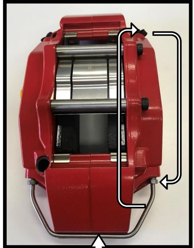
🇬🇧 The bottom brake pipe and the bleeding screws can or need to be swapped from top to bottom or vice versa depending on the application
