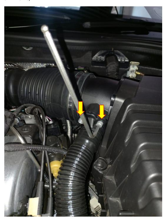
5. The OEM Plastic pipe and flanges can now be removed from Situ.
