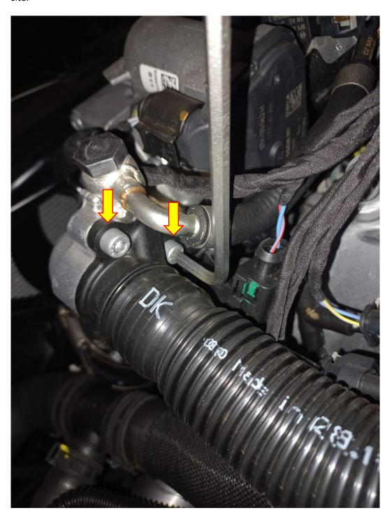
4. Following the plastic pipe to the opposite end remove the flange from the intake using a 5mm Allen key.
