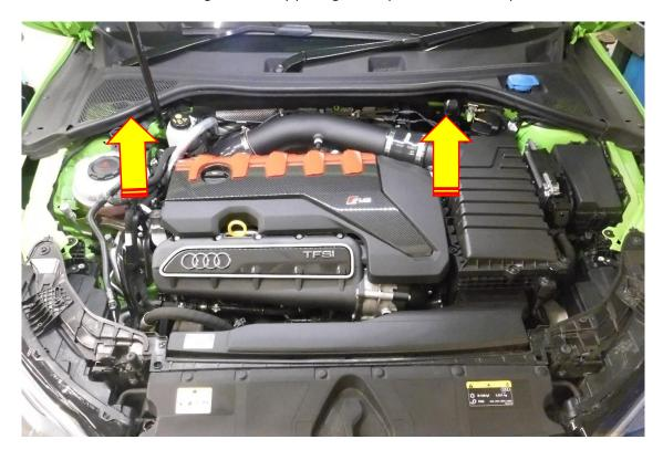
2. Locate the dump valve elbow as arrowed below.
