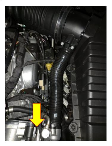
3. Using a 5mm Allen Key Remove the fasteners that hold the Dump valve recirculation tube in situ.
