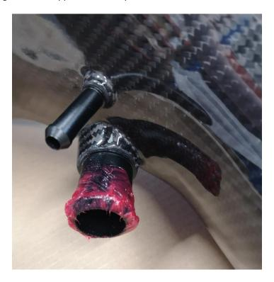
**10.** Now fit the Forge silicone hose and hose clamps provided using a 7mm hose clamp drive or suitable tool tighten the hose clamps in situ.
