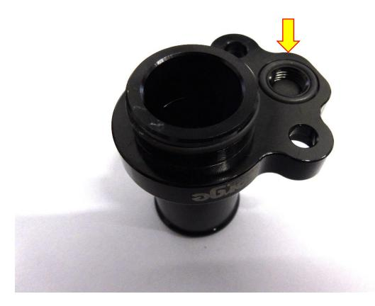
7. Using a 5mm Allen key tighten the supplied Allen cap head bolts into position.
