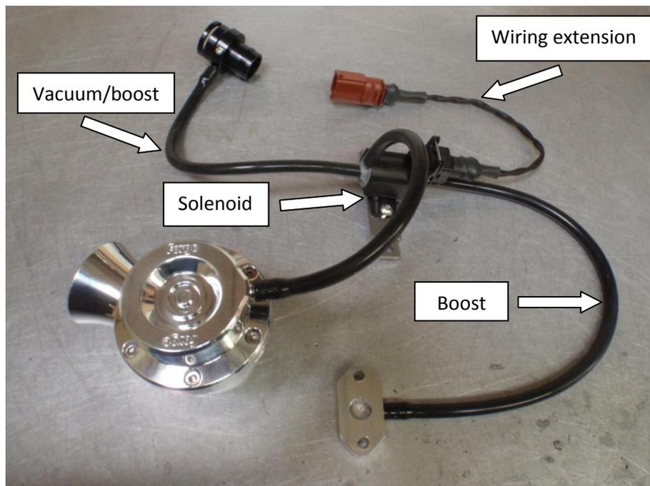
7. Please note the position of the wiring extension and direction of the vacuum take off on the BOV.
