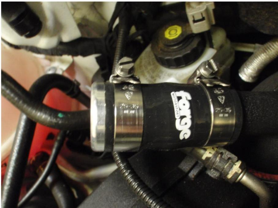
9. Forge motorsport highly recommend venting to atmosphere as this valve has a bigger bore for releasing the boost pressure. However you can install this valve recirculating if you wish. Screw in the small tube supplied in the kit and reattach the stock hose. Follow step one in reverse order and your installation is now complete.
