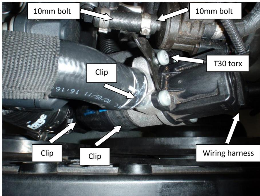
2. Unclip the breather and install the PCV take off, the take off should have two of the holes blocked off with grub screws unless you wish to fit a boost gauge etc. The other hole needs a vacuum take off with the largest hole screwed in. Secure the PCV take off with the small plastic clip supplied in the kit.
