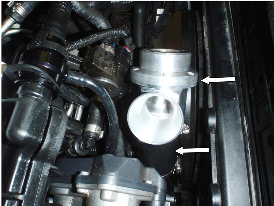
6. The photo below shows how to install the vacuum hoses and wiring extension. When installing in the car, the vacuum hoses and wiring extension can be routed under the inlet manifold for a neat installation.
