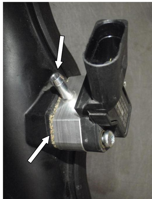
5. Install the silicon hose and BOV with the clips supplied in kit.
