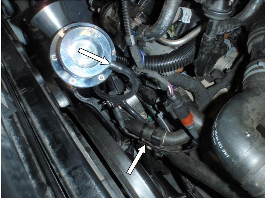
8. For venting to atmosphere at the back of the engine bay install the silicon hose, bung and clips supplied in the kit onto the filter pipe.
